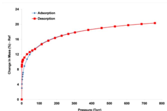
13X adsorption-desorption of CO<sub>2</sub> in the pressure range from 0 to 760 Torr at 25°C. 13X was in the form of beads having 1-2mm diameter.
