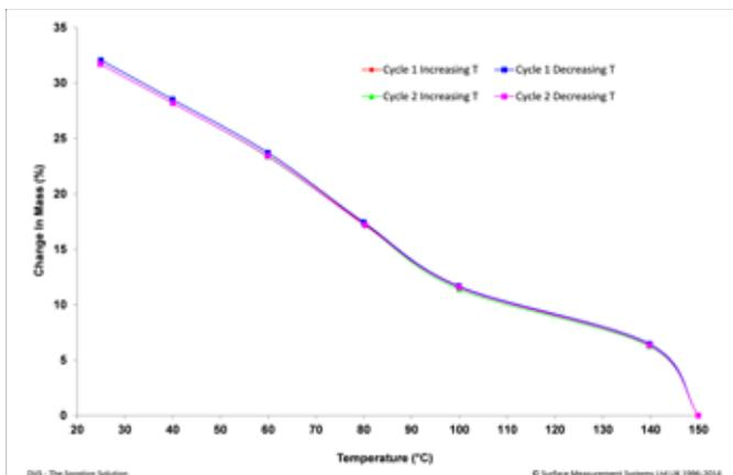
A10 water vapor isobars at 7.14 Torr (Figure left). Two cycle of A10 showing change in the mass (in red) during stepping down (adsorption) and stepping up (desorption) temperature (in blue) at pressure (in green) of 7.14Torr. A10 water vapor isobar at 7.14 Torr (Figure right).
