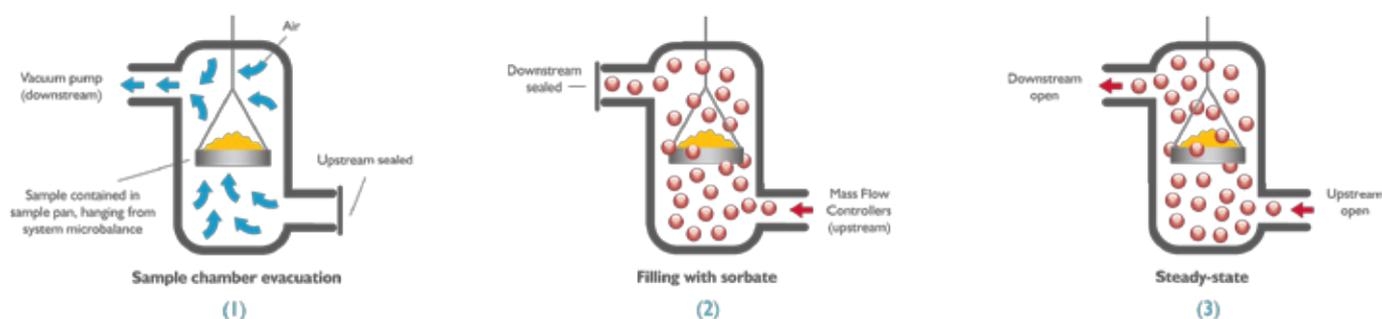
1. *In-situ* degassing of sample under high vacuum and high temperature. Downstream consisting of butterfly valve controlling pumping speed is fully open, while upstream controlled by mass flow controllers is closed.
