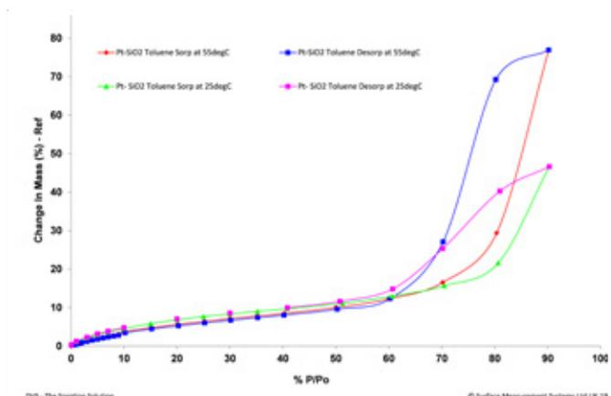
Comparison of Pt-SiO<sub>2</sub> toluene adsorption-desorption isotherms at 25 and 55°C (left). Determination of specific surface area using BET equation for toluene sorption at 55°C (right).
