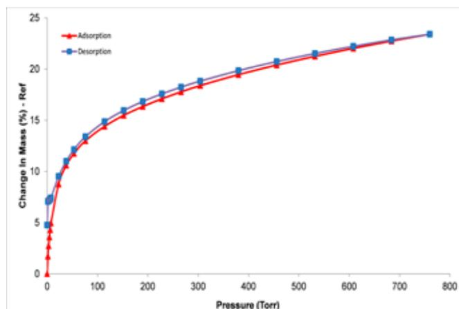
Mg-MOF-74 adsorption-desorption of CO<sub>2</sub> in the pressure range from 0 to 760 Torr 25°C.
