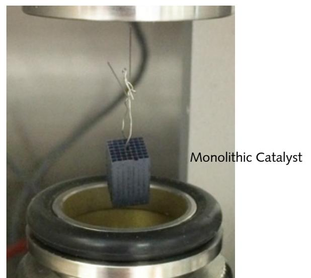
Variable samples such as catalytic converters, thin films and porous membranes can be measured in the system. The sample is connected directly on the hangdown wire. In typical experiments, where powders, pellets or beads are used, samples are loaded in stainless steel pans. Other experimental cells are available for a wide range of sample types and applications such as diffusion/permeation and Knudsen vapor pressure.
